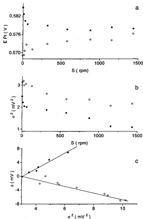
**Figure 1.** Dependence of the system response on stirring rate: (a) time average of the Pt-electrode signal and (b) its variance. Panel (c) gives the linear relationship between the shift  $\Delta = E_{Pt}(S) - E_{Pt}(1500)$  and the variance  $\sigma^2$ . Open circles – NPM mode, closed circles – PM mode.
