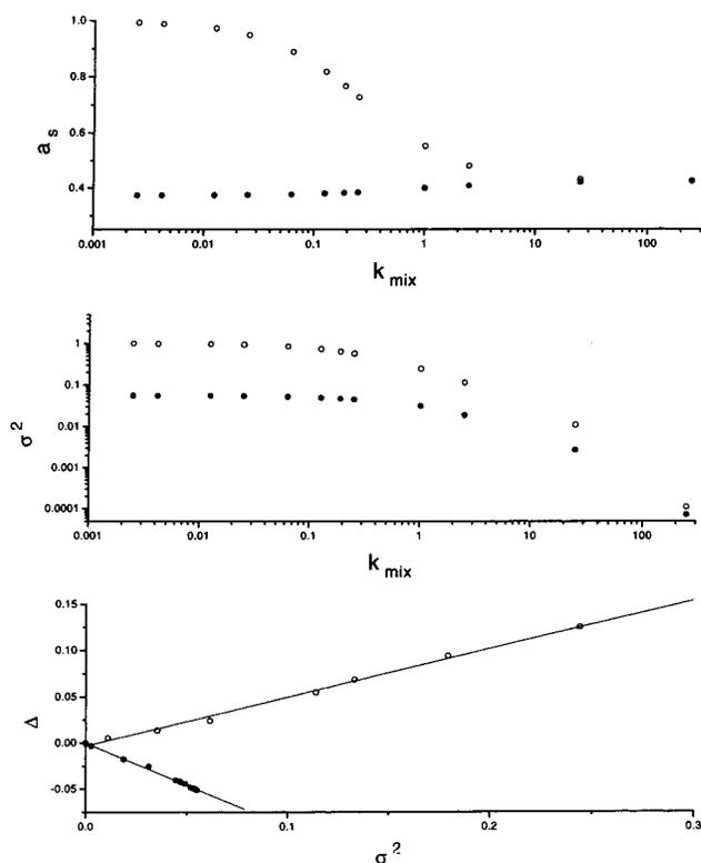
**Figure 2.** Dependence of (a) the average reactant concentration ( $a_s$ ) and (b) its variance on the mixing rate, obtained by simulations for the bimolecular reaction  $A + B$  in a CSTR ( $[A]_0 = [B]_0 = 1$ ;  $k = 0.4$ ,  $k_0 = 0.125$ ). Panel (c) illustrates the linear relation between the shift  $\Delta = a_s - a_d$  and the variance  $\sigma^2$  for both PM and NPM modes. Symbols as in Figure 1.
